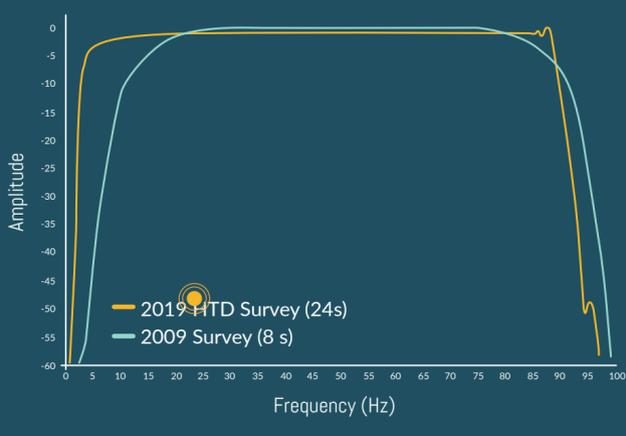
Because HTD acquisition designs combine high fold with a small bin size, they enhance the signal-to-noise ratio and reduce the noise floor, improving vertical and lateral resolution. The increased acquisition of near-offsets enhances the resolution of shallow events.
